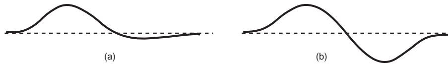
Fig. 9. Schematic representation of primitive modeshapes from the two B-spline model: (a) homoclinic ( Q_1 \neq -Q_2 ); (b) periodic ( Q_1 = -Q_2 ).
